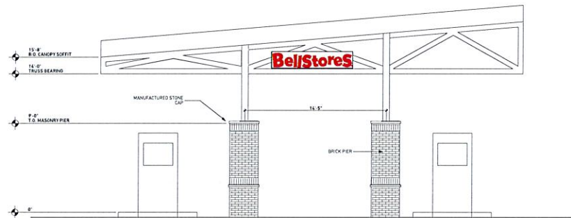
C1 FUEL CANOPY ELEVATION - NORTH SCALE 1/2" = 1'-0"
